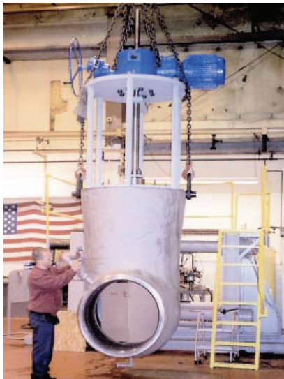
36” Class 705 SPL INT Parallel Slide Gate Valve WT – 25,300 lbs. 15 ½ Ft. Tall
